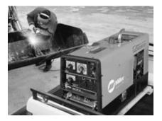
**PipePro 304:** With its patented weld-at-idle feature while welding at 150 A at 40% duty cycle using 5/32 in. 7018 electrode, the PipePro averaged 0.4 gallons per hour.
