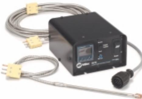
The Miller IH/TC is a temperature control package designed specifically to interface with the IHPS™ II and Intellifire™ power sources. The single-station controller processes temperature feedback from a single thermocouple sensor and adjusts power source output to regulate or maintain part temperature. The IH/TC is supplied with a temperature sensor, sensor extension cable and interconnect control cord for use with the induction heating systems.
