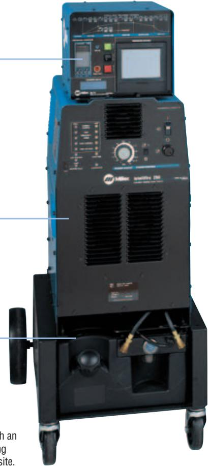
The Intellifire 20 and 25 kW Systems can be equipped with an optional lifting eye for moving the system at a construction site.
