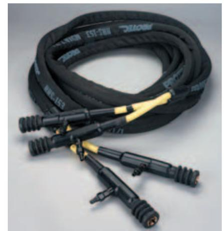
The cable is equipped with Twist-Lock quick disconnects for easy removal and attachment. Liquid-cooled extension cables are available to remote the power source up to 50 feet from the work. The cables are flexible for ease of use.
